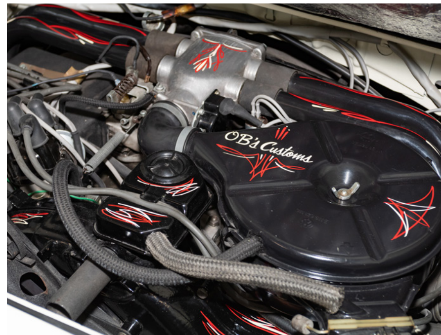
Completely stock 1600cc with original fuel injection remains in place. “I spent a lot of time learning to maintain the system”, says Spencer.
