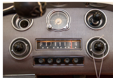
1951 stock Ford radio, which has been converted to digital output.
